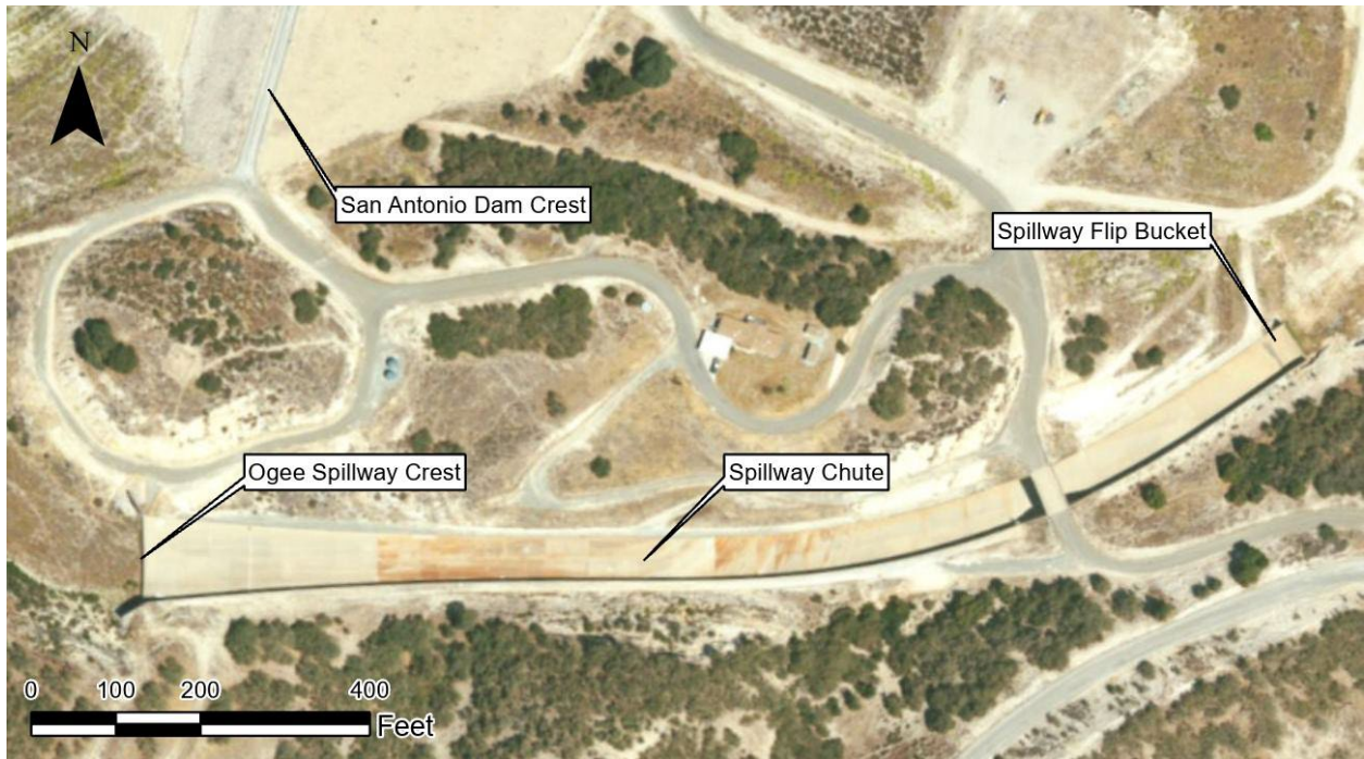
Figure 2: San Antonio Dam Spillway Alignment
