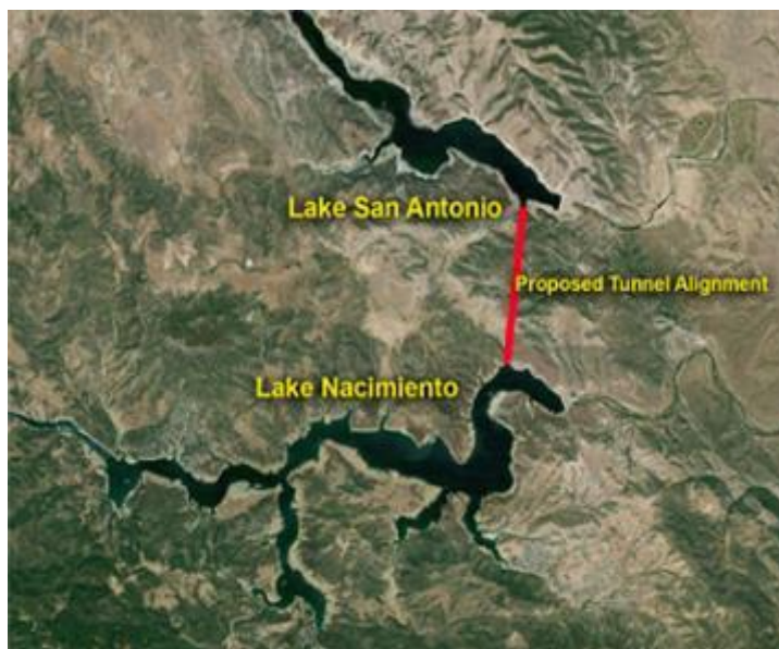
Figure 18: Proposed approximate tunnel alignment.
